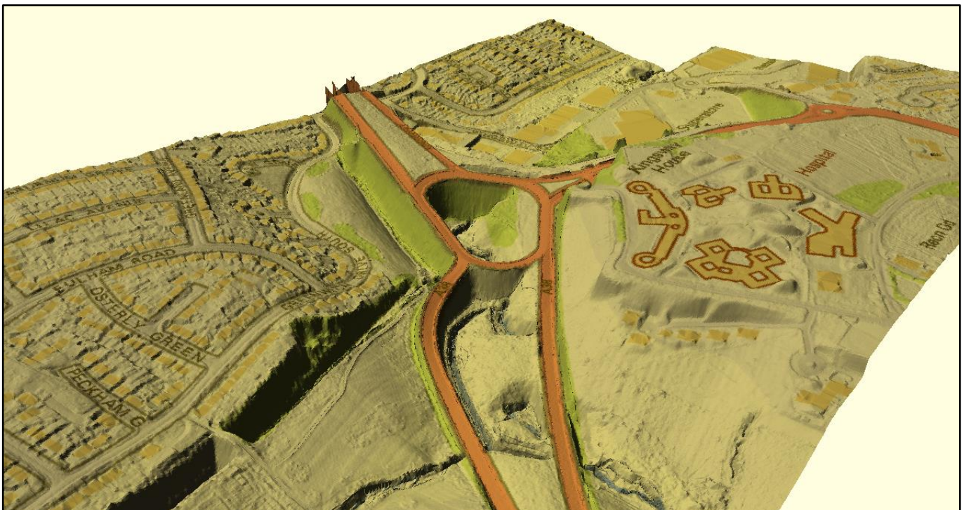
Figure 3: Representation of the existing Kingsway junction based on the modified ground model (incorporating topographic survey with the LiDAR as a TIN ground model)
